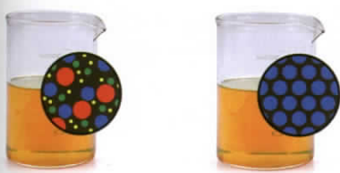
Mineral oils are made up of a range of various sized molecules. Full synthetic base oils are highly refined by man-made processes to yield uniform molecules in ideal quantity.
