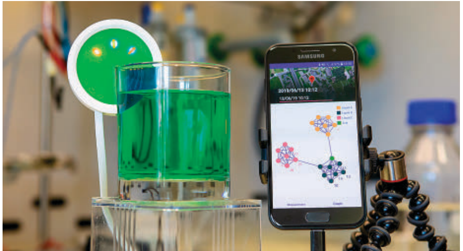
The smartphone displays the results of Hypertaste, an AI-assisted “tongue” app from IBM Research that uses electrochemical sensors to analyze complex liquids.
