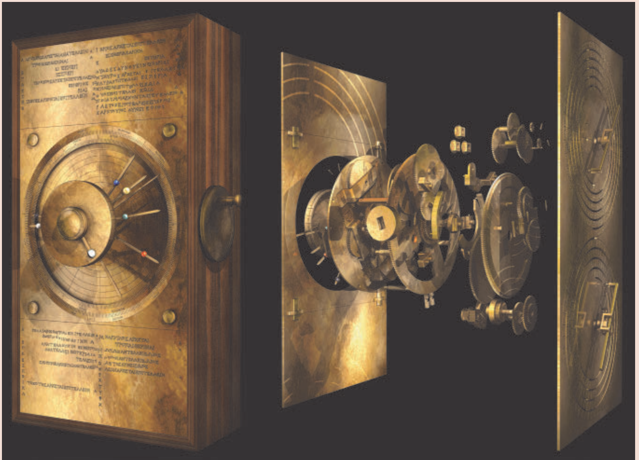
Figure 6. Digital reconstruction by Tony Freeth: on the left the front side with the two concentric scales and seven pointers, on the right the back side with the spiral scales, among others for the display of solar and lunar eclipses (courtesy of Tony Freeth, Images First Ltd., London).
