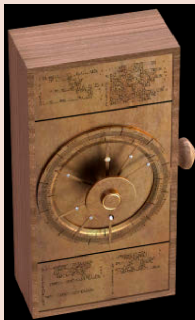
Figure 2. The front of the Antikythera Mechanism shows seven hands (sun, moon, five planets) and a double ring scale (outside: Egyptian calendar, inside: zodiac). At the top and bottom of the digital model is the Parapegma inscription (courtesy of Hublot, with data from the Antikythera Mechanism Research Project).
