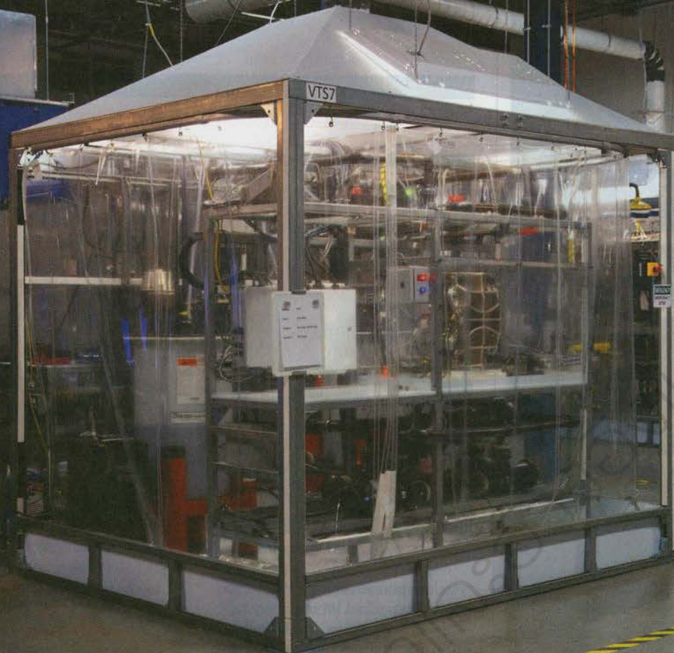
LIQUID ASSETS A device used to test Vionx's flow batteries, which rely on tanks of chemicals to help store energy.
