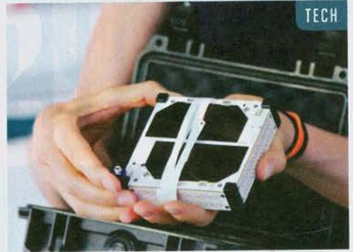
One of the tiny satellites that startup Swarm plans to use in its space-based broadband network.
