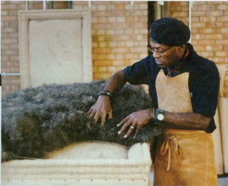
A craftsman fills the mattress with South American horsetail hair [left]. A Savoir Beds mattress is "tufted" (right) to prevent the filling from moving.
