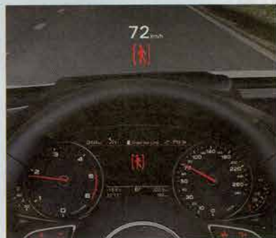
▲ The driver assistance system in the Audi Q7 has a night vision feature to help prevent hitting pedestrians.
